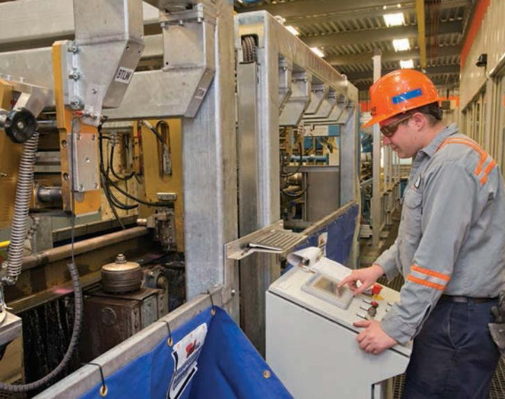
Quality control improvements with additional nondestructive testing (NDT) enhance flaw detection. The NDT station also improves safety. Because the entire finishing end now is communicating over one Ethernet network, EVRAZ can create system alerts for operators that are useful for situations such as preventing rails from colliding with one another.
